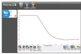
The graph shows the measurement of the oxygen logger sensor while inside the combustion environment. It can be seen that the initial free oxygen measurement is about 21% as it should be in the atmosphere; the concentration decreases to about 15% when the candle goes out. This result is far from the one expected by students.
