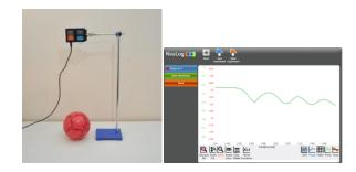
The graph demonstrates the motion of a bouncing ball by using a motion logger sensor pointing down. When the ball bounces back up, it reaches a height that is less than its original height due to energy loss.
