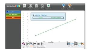
The graph demonstrates Ohm's Law: the current is proportional to the voltage. The slope of the graph is the resistance.
